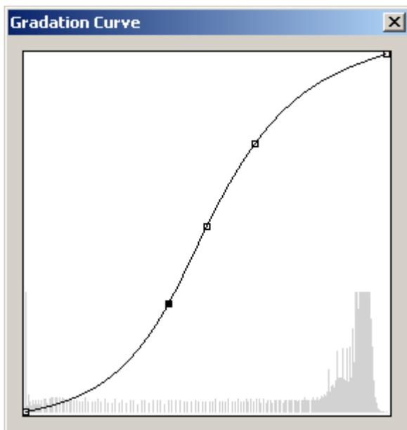
**Figure 88: RGB-gradation curve with 3 supporting points**
