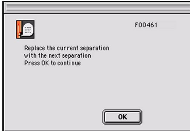
3. Remove the first separation and mount the second one inside the cell size you defined for the first separation. Then close the top cover.
